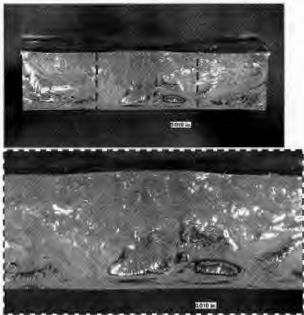
Figure 5 – Fracture surface of a polycarbonate sample after exposure to biodiesel and 1.5% strain.
